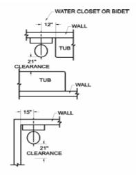
FIGURE 307.2 MINIMUM FIXTURE CLEARANCES
